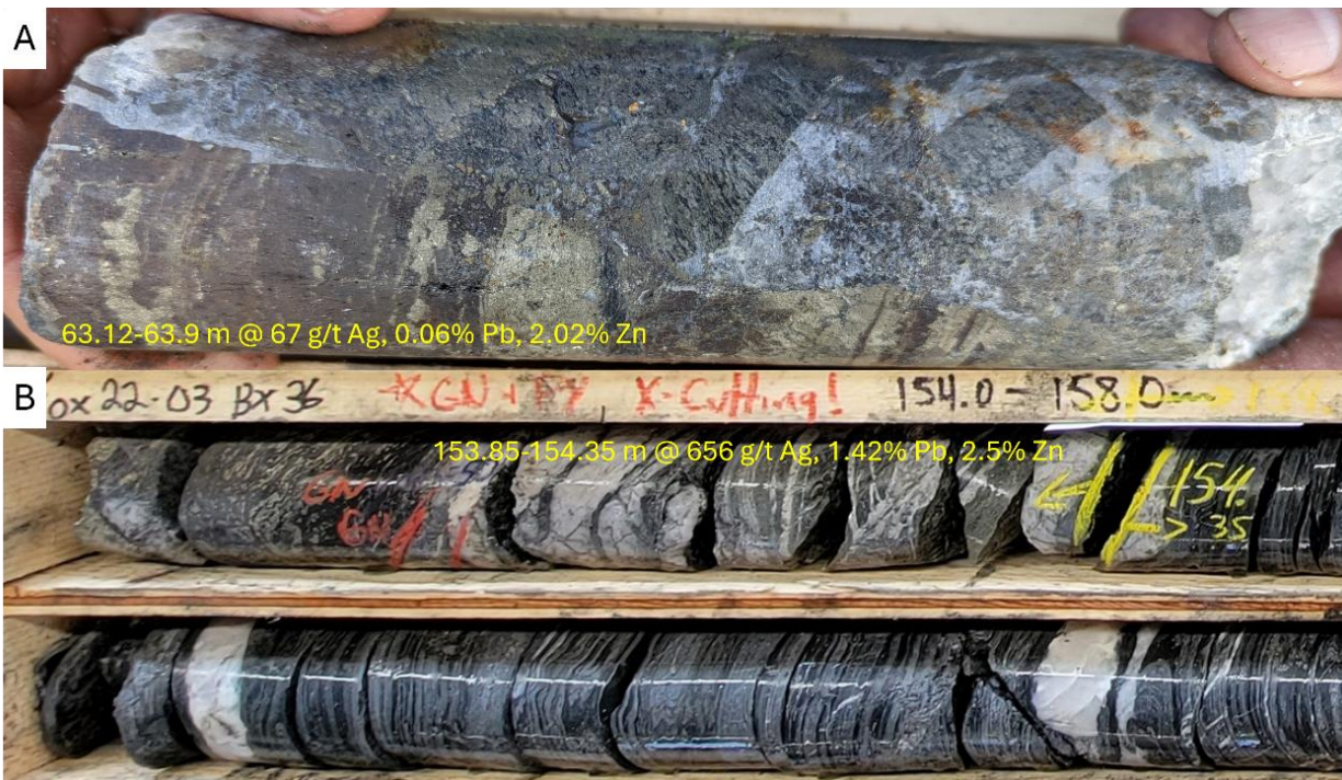
A) Discordant vein mineralization hosted within greenstone primarily as sphalerite and pyrite with a brecciated quartz carbonate gangue; B) Discordant vein mineralization hosted within the graphitic schist primarily as argentiferous galena and sphalerite with quartz carbonate gangue.
