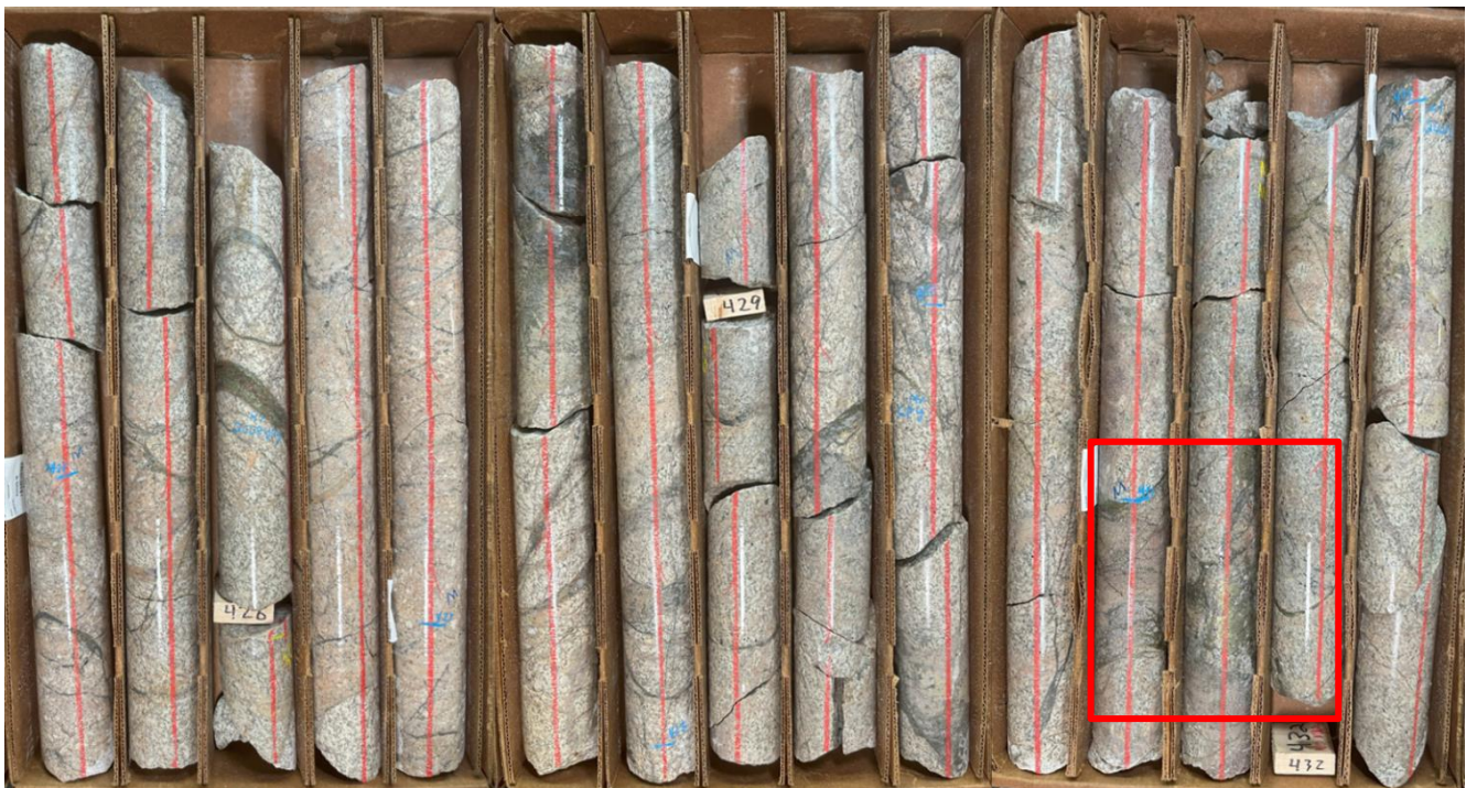
Figure 3 – Core photos of Hole LAP23-05 from 425 m to 433 m showing an example of strong porphyry style mineralization including multi-phase veining and strongly disseminated copper sulphides.
