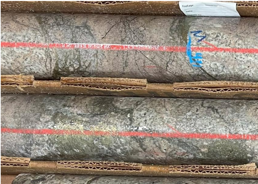
Figure 4 – Core photo detail of from red outline above in Figure 3 showing the intensity of copper sulphides including chalcopyrite and bornite.
